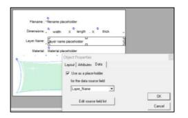
• XY 0 ,0 Guide lines checkbox at plate creation We have added a checkbox to create XY-guidelines at the origin of the plate upon its creation.
